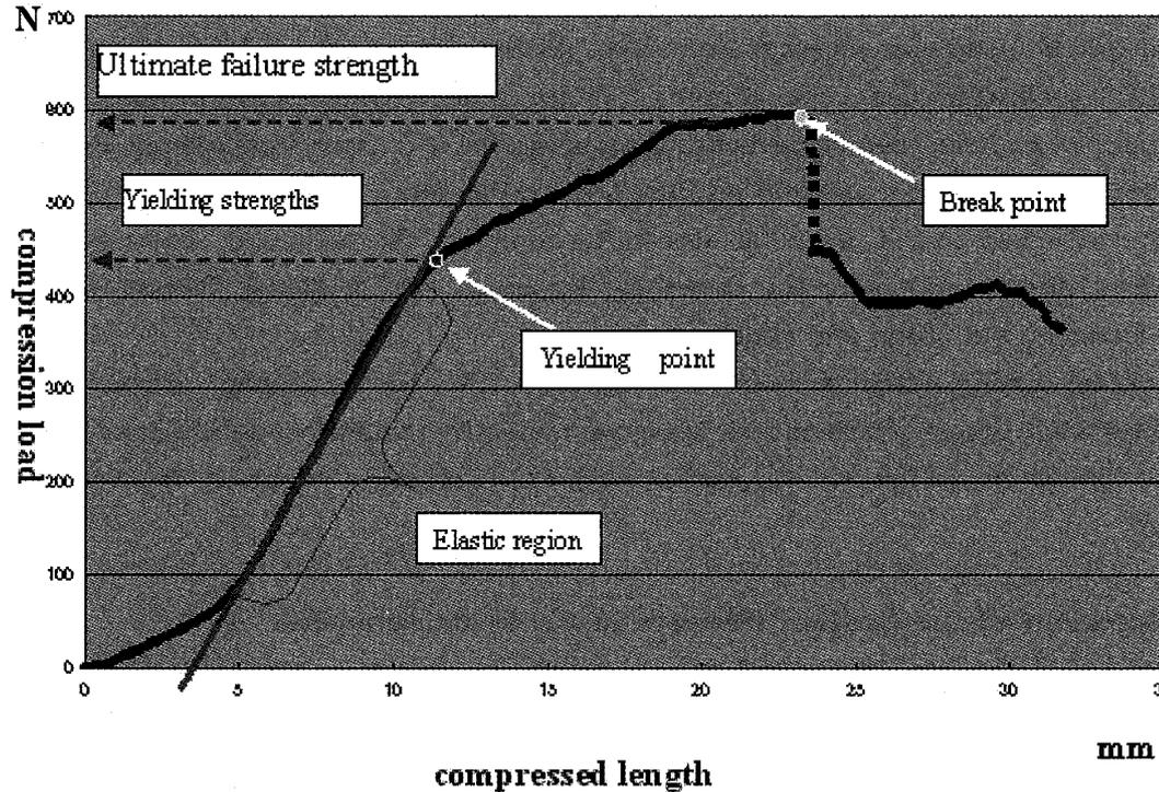
Fig 2 : Stress-Strain curve.
